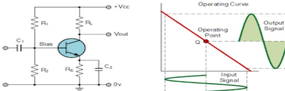
To achieve high linearity and gain, the output stage of a class A amplifier is biased “ON” (conducting) all the time. Then for an amplifier to be classified as “Class A” the zero signal idle current in the output stage must be equal to or greater than the maximum load current (usually a loudspeaker) required to produce the largest output signal.
