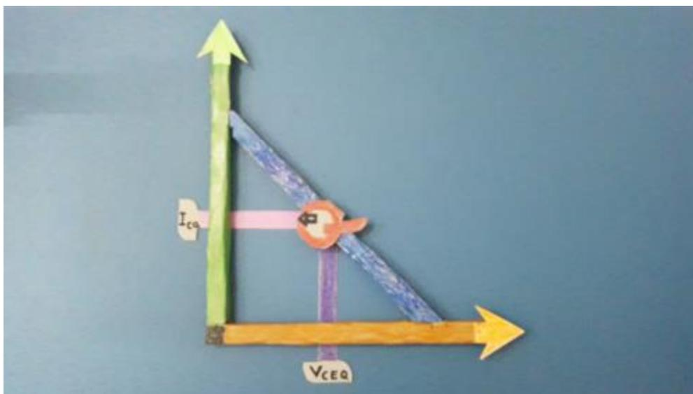
The above model shows the load line with Q point at its centre.  $V_{(CEQ)}$  is pretty much the same as  $V_{(CE)}$  in terms of its behaviour, with the only difference being that it's more of a specific kind of value than rather being a range of values. The same is true for  $I_{(CQ)}$  and  $I_{(C)}$  as well.
