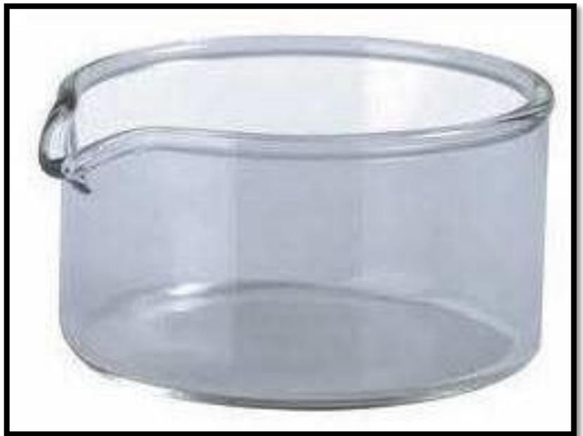
*Figure 1.13 Crystallization dish*
