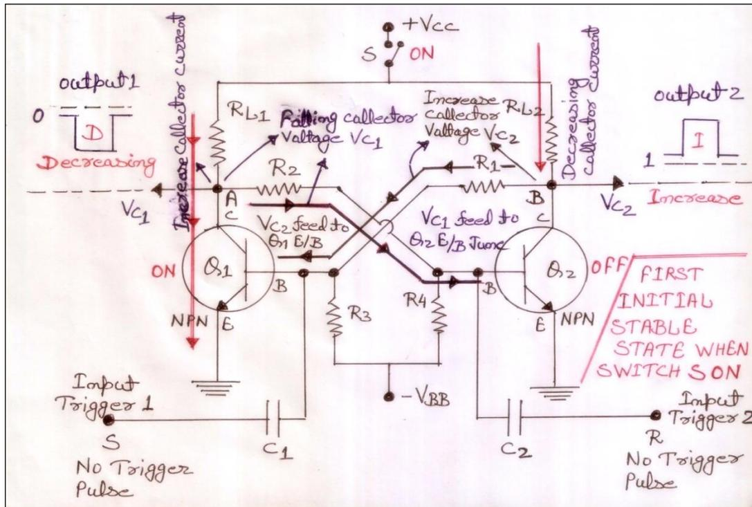
Fig. (3) Shown First Initial stable State of the Multivibrator when BMV Power Switch 'S' ON and No Trigger Inputs applied.
