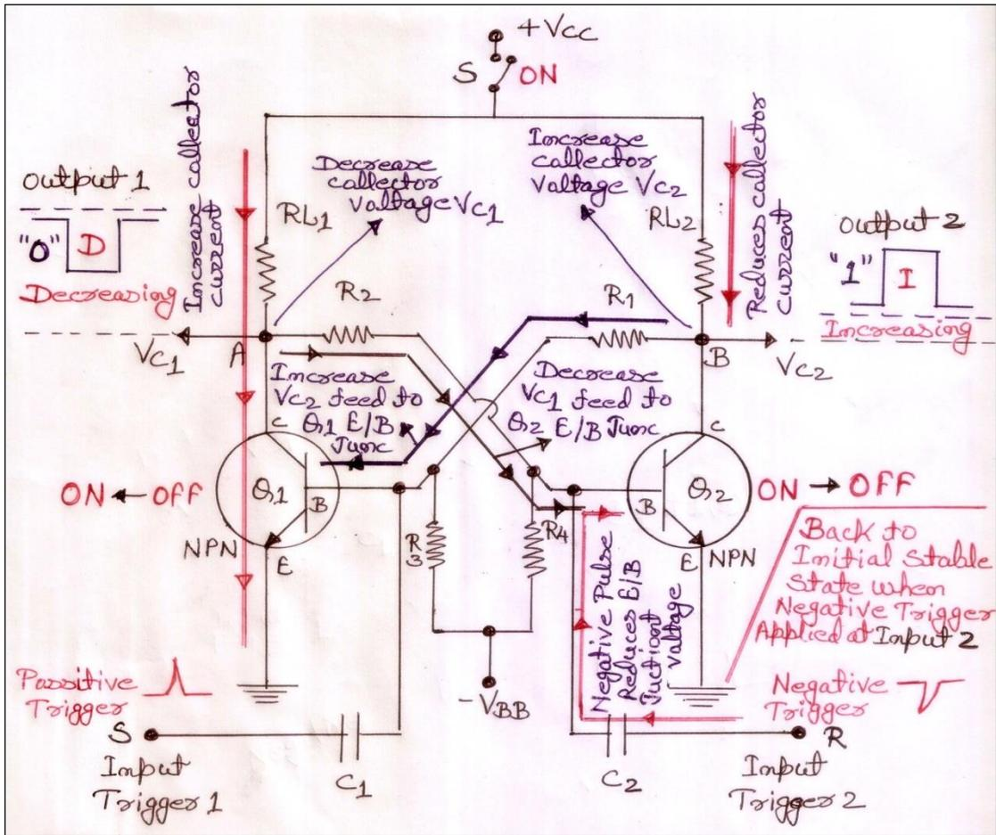
**Fig. (5)** Shown Back to initial stable state of BMV can be achieved when negative trigger pulse applied to the transistor Q2 through Input 2 or Positive trigger pulse applied to the transistor Q1 through Input 1.
