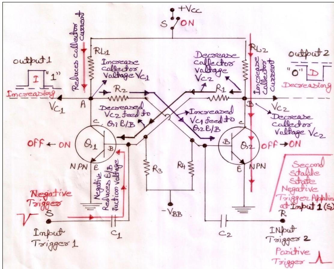
Fig. (4) Shown Second stable state when negative trigger pulse applied to the transistor Q1 through Input 1 or Positive trigger pulse applied to the transistor Q2 through Input 2.
