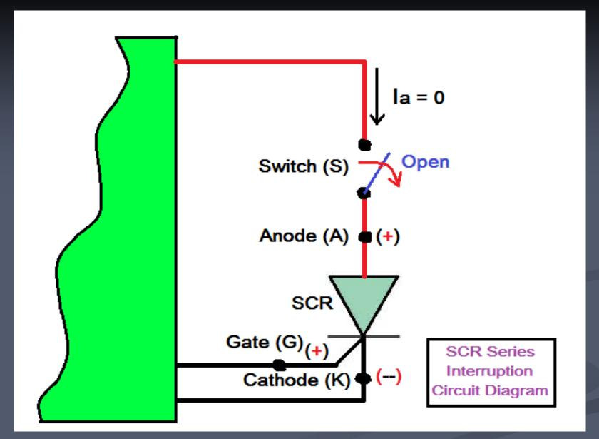
Fig (77) Shown a Series Interruption Technique in which Anode Current (Ia) of SCR is interrupted to become Zero when the circuit Switch S is Opened.
