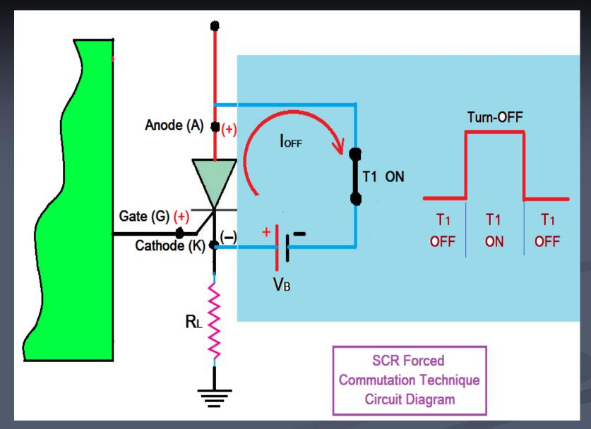
Fig (80) Shown a Basic Type of Force Commutation Circuit Diagram using NPN Transistor and a Battery for applying Reverse Biasing across SCR.
