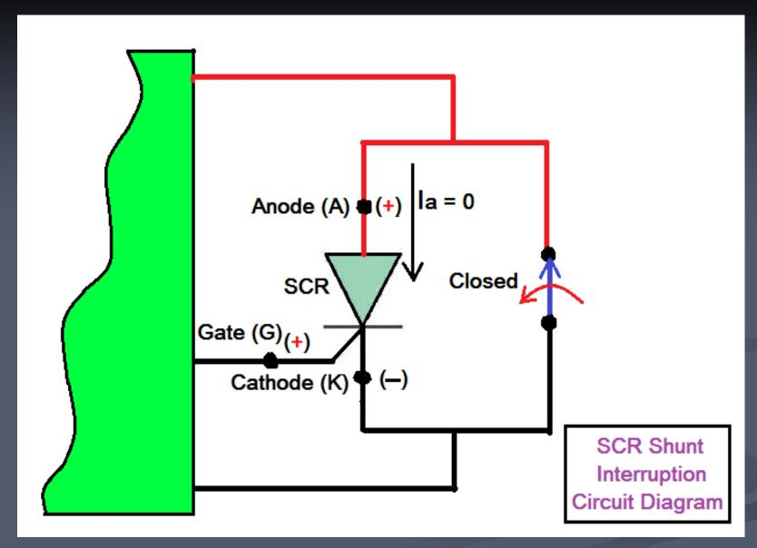
■ Fig (78) Shown a Shunt Interruption Technique in which Anode Current (Ia) of SCR is interrupted to become Zero when the circuit Switch S is Closed.
