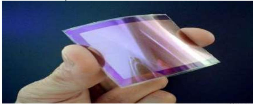
New solar panel films incorporate nanoparticles to create lightweight, flexible solar cells. (Image courtesy of Nanosys)
