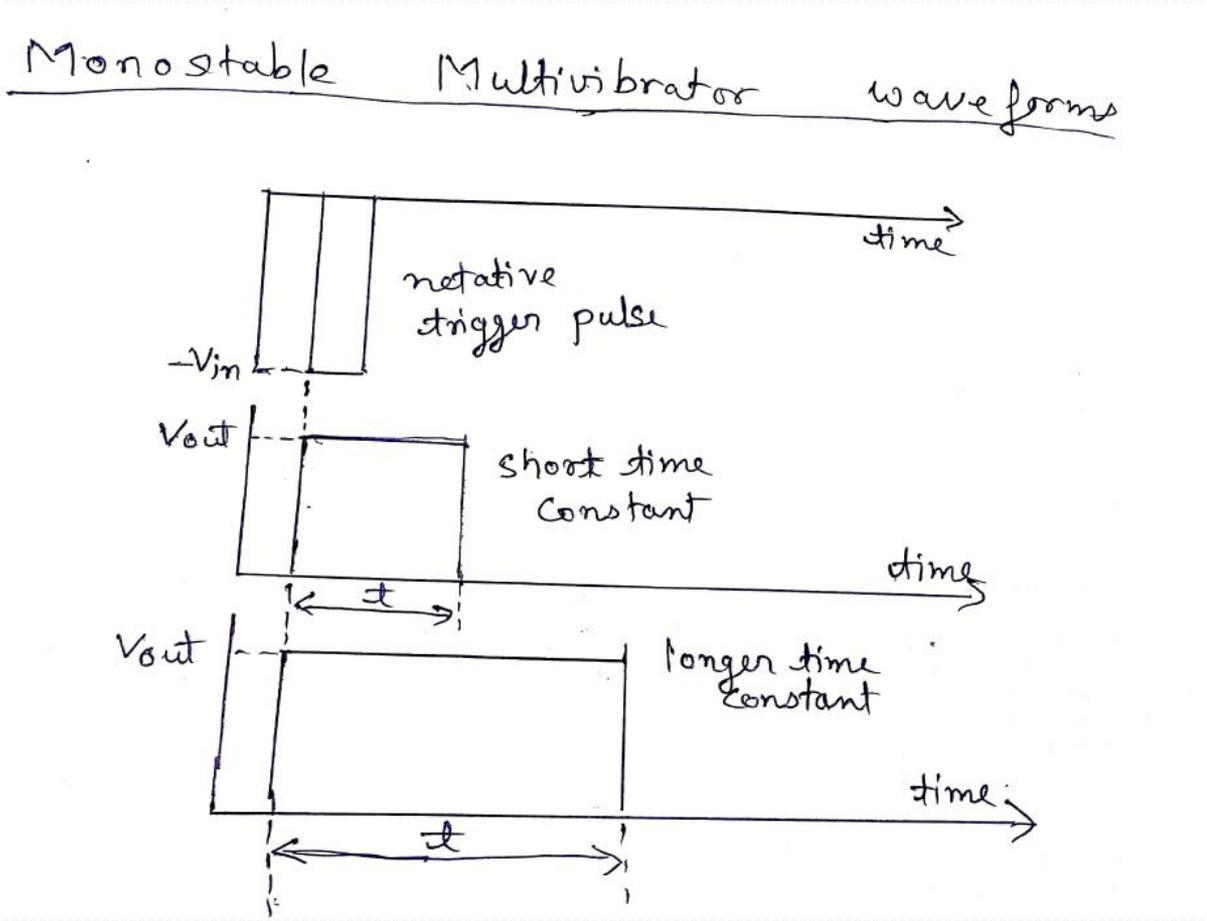
The time constant of monostable multivibrators can be changed by varying the values of the capacitor and resistor or both. Monostable multivibrators are generally used to increase the width of a pulse to produce a time delay within a circuit as the frequency of the output signal is always the same as that for the trigger pulse input, the only difference is the pulse width.
