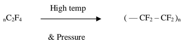
Teflon has a low coefficient of friction. It is thermally and chemically inert and a good insulator. It is used as a coating material in non-stick utensils, razors and bearings.
