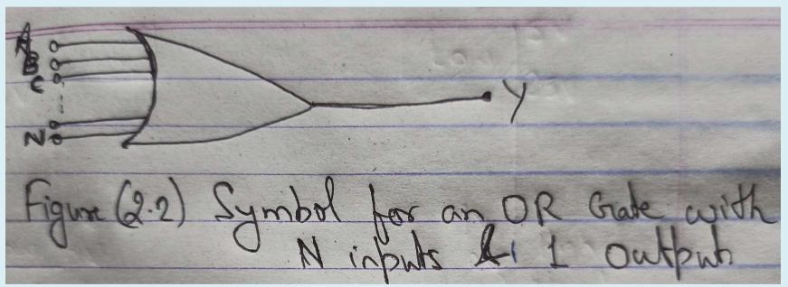
Operation of an OR Gate with any numbers of inputs can be shown through its truth table.
