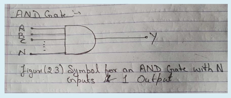
Operation of an AND Gate with N numbers of inputs can be shown through its truth table.
