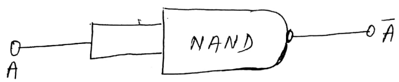
Fig. 6(a) NOT-gate from NAND gate.
