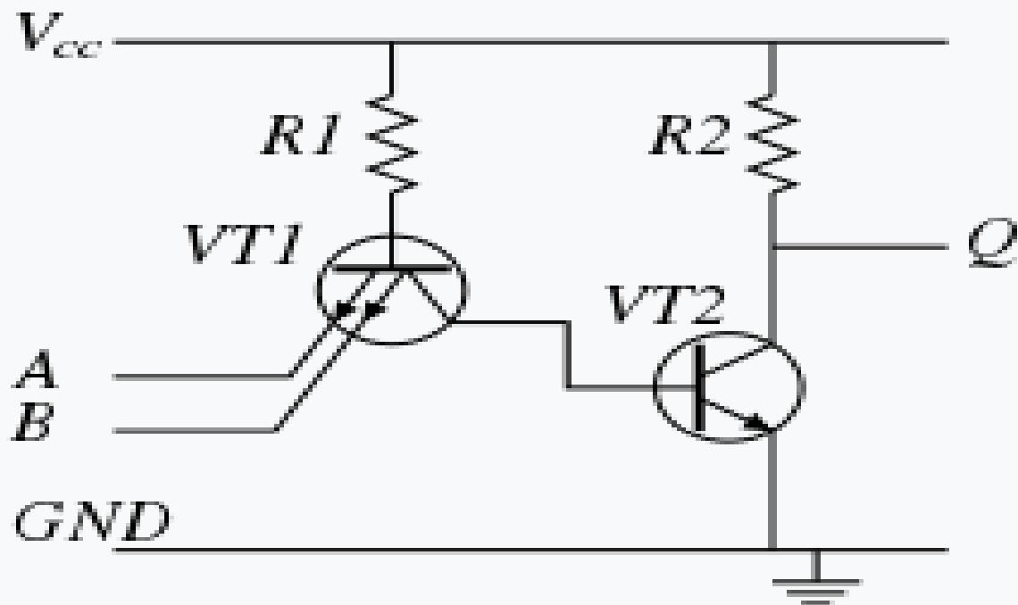
**Two-input TTL NAND gate with a simple output stage (simplified)**
