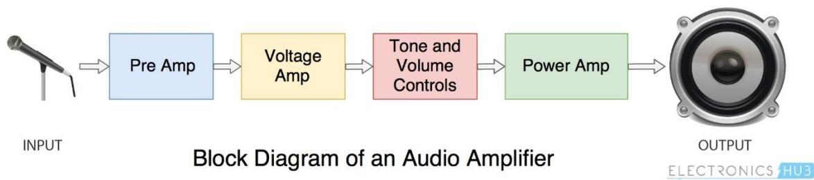
In this case, a microphone is used as an input source. The magnitude of signal from the microphone is not enough for the power amplifier. So, first it is pre-amplified, where its voltage and current are increased slightly. Then the signal is passed through a tone and volume control circuit, which makes aesthetic adjustments to the audio waveform. Finally, the signal is passed through a power amplifier and the output from power amp is fed to a speaker.
