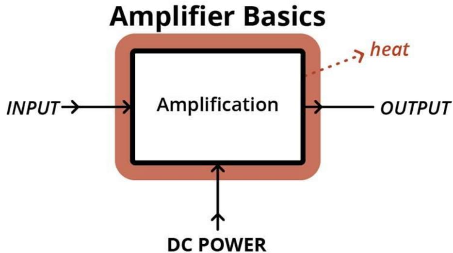
**Amplifier Class** is the system for combining power and signal. Amp class differs from amp to amp with efficiency and sound fidelity dependent on which design gets used. In all designs, banks of output transistors, each a little amp by itself, add their collective power together to provide the amplifier's final output.
