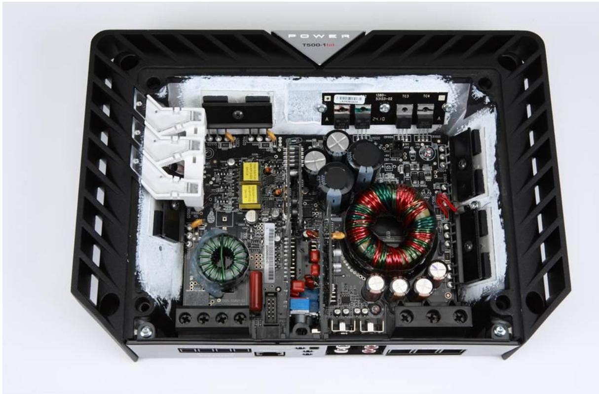
The inside of a [Rockford Fosgate T500-1bdCP](#) showing the transformer (the coil of red and green wires) and output transistors (black rectangles glued to the heatsink with white thermal paste).
