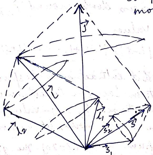
In L-S coupling (fig) the individual orbital angular momentum vectors  $\vec{l}_1$  and  $\vec{l}_2$  of two electrons are strongly coupled to each other to form a resultant orbital angular momentum
