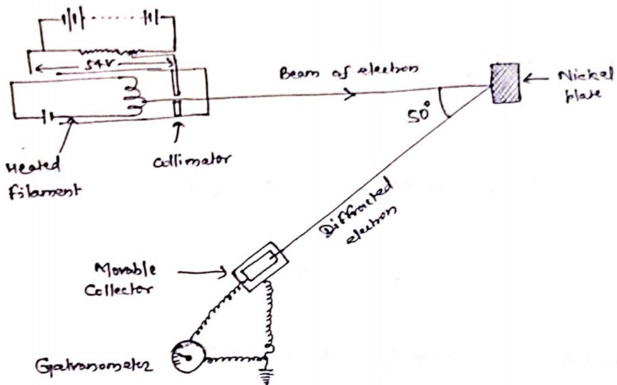
The impact of electrons resulted in the production of diffraction patterns which were similar to those of X-rays under similar conditions. Since, X-rays possess wave character, the experiment gave direct evidence for wave character of electron as well.
