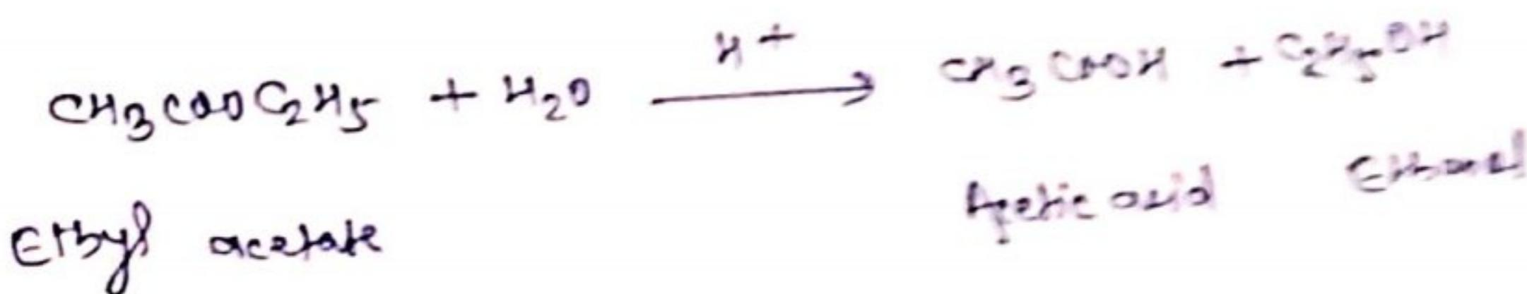
$$\text{Here, Rate, } \propto = K [CH_3COOC_2H_5]^1 [H_2O]^0$$
